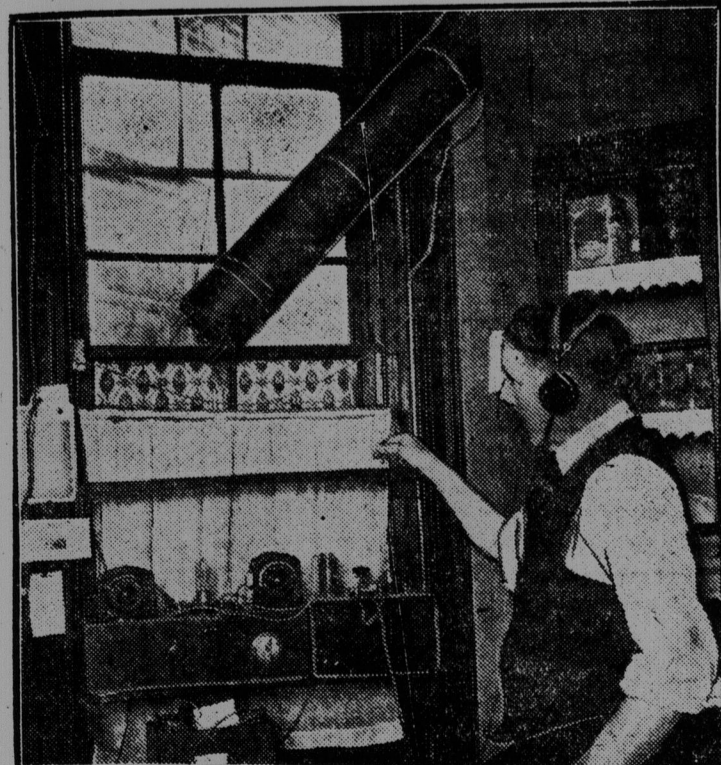
When Edward Kelly, a New York tenement dweller, stopped from erecting an aerial on the roof, he got over difficulty by using a few lengths of stove pipe.
