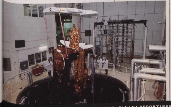
in the world capable of simulating launch conditions and space environments on satellites up to 4 500 kg, the laboratory provides a vital service for domestic industries as well as foreign agencies. It played a critical role in the success of the Canadarm. Sweden's Viking, and the SARSAT search-and-rescue satellite developed jointly by Canada, the United States and France. Currently, the European Space Agency's largest and most complex satellite, the Olympus, is undergoing tests at the facility.
