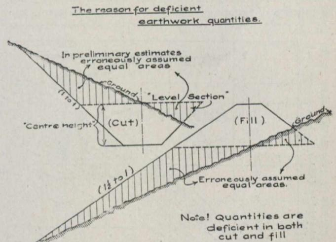
FIG. A—Effect of Changes of Surface Slope on Area of Cross-Section.
