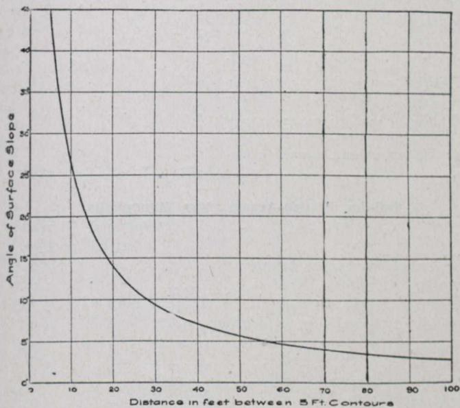
Fig. C—Relation Between Angle of Surface Slope and Horizontal Distance Between 5-ft. Contours.
