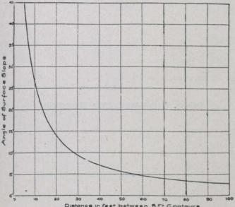
Fig. C—Relation Between Angle of Surface Slope and Horizontal Distance Between 5-ft. Contours.
