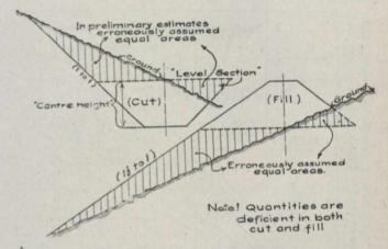
Fig.A—Effect of Changes of Surface Slope on Area of Cross-Section.
