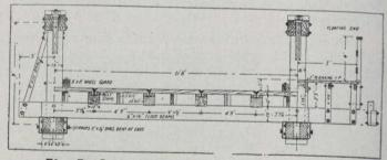
Fig. B-Cross Section at Floating End of Span.
