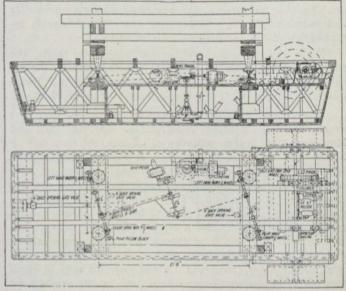
Fig. D—Plan and Section of Scow Showing Arrangement of Machinery.
