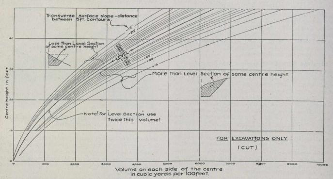
Fig. B-Effect of Changes of Surface Slope on Volume of Earthwork. Base 20 ft.; Slope 1 to 1.
