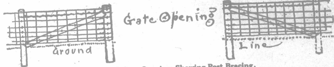
Fig. 3—A Gate Opening, Showing Post Bracing.
