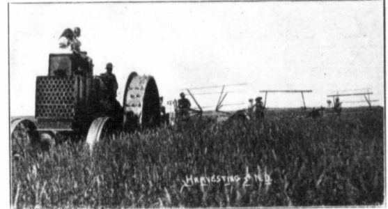
A Gas Traction Operating Binders by means of a Hansmann Binder Hitch
