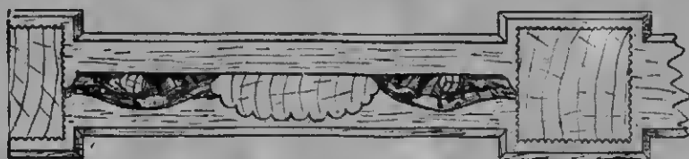
Fig. 1795.—Horizontal Section through Communion Rails at level of A (Fig. 1787).
