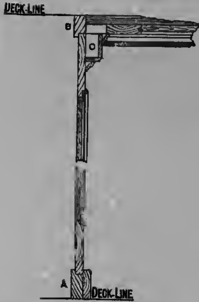
Fig. 1906.—Vertical Section of Ship's Ventilator Cover.
