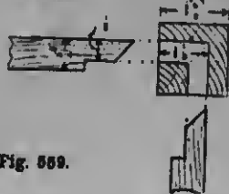
Fig. 556 and 559.—Joint of Rail and Leg of Dressing Table.
