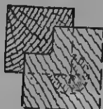
Fig. 51.—Shelf Housed to Leg of Table.
