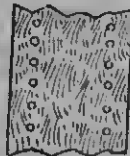
Fig. 737.—Holes in Side of Cabinet-bookcase to receive Movable Shelves.
