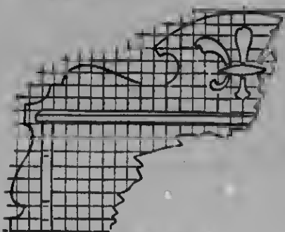
Fig. 294.—Pattern for Shaped Back of Cabinet Bookcase.
