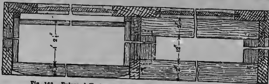
Fig. 163.—Enlarged Horizontal Section through Drawers of Sideboard.
