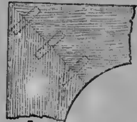
Fig. 1525.—Joint of Shelf in Cozy Corner Settee.
