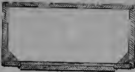
Fig. 1987.—Horizontal Section of Grandfather Clock Case at A (Fig. 1985).
