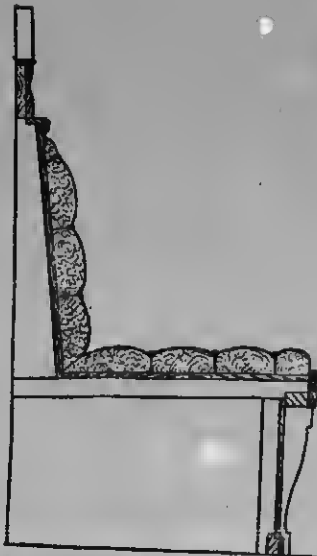
Fig. 1917.—Vertical Section of Sofa.
