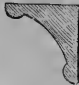
Fig. 1522.— Bracket for Legs of Cozy Corner Settee.
