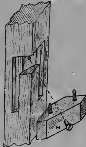
Fig. 1389.—Housing in Palm Stand Leg for Shelf Rails.
