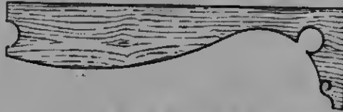
Fig. 640.—Half of Bedstead Bracket Piece.
