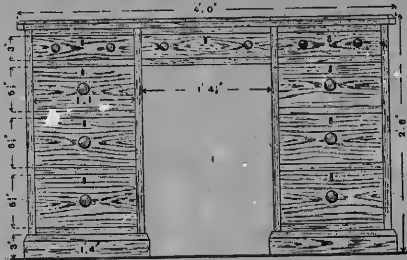
Fig. 782.—Front Elevation of Pedestal Writing-desk.
