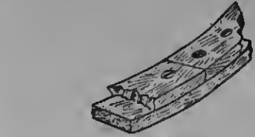
Fig. 1635.—Two Thicknesses Lapped to form Frame.
