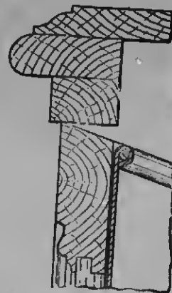
Fig. 429.—Nosing, etc., of Chief Shelf of Coal Cabinet (C, Fig. 425).
