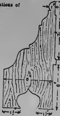
Fig. 1656.—Mirror Support for Shaving Stand.
