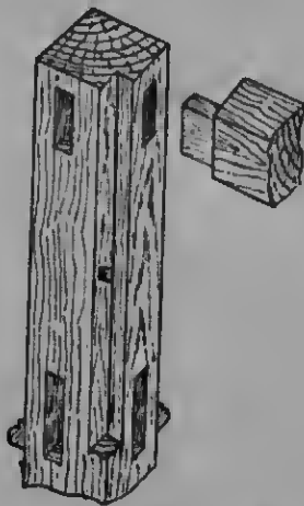
Fig. 1497.—Joint in Curio Table.
