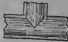
Fig. 486.—Plan of Umbrella Stand's Top-rail Joint.
