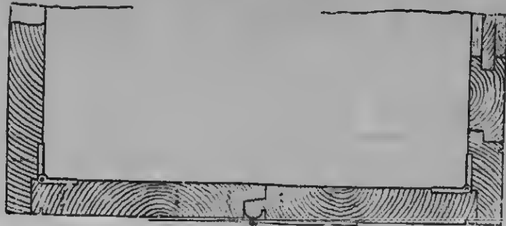
Fig. 1151.—Part Horizontal Section of Collapsible Cupboard.
