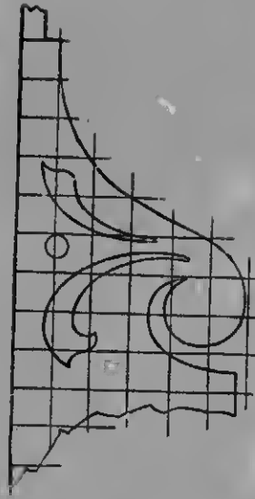
Fig. 352.—Pattern for Part of Cabinet Back.
