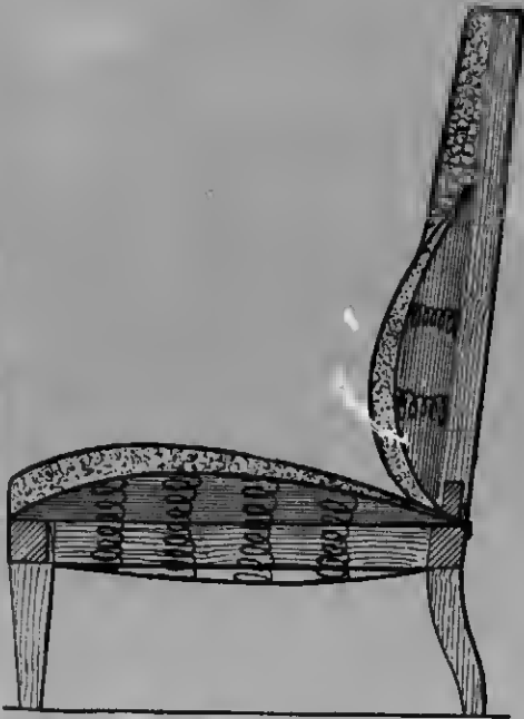
Fig. 97.—Vertical Section of Easy Chair showing Springs and Upholstery.
