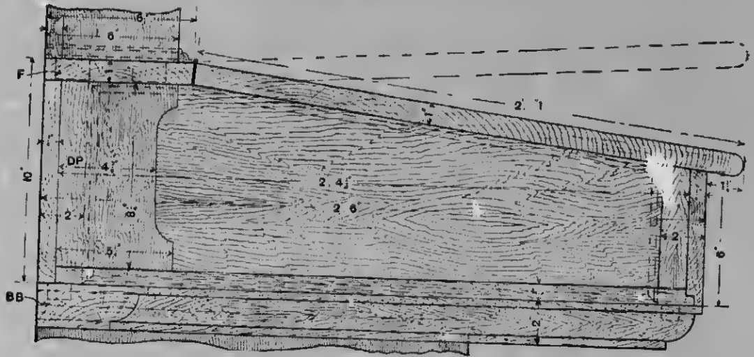
Fig. 883.—Part Vertical Section of Portable Desk.
