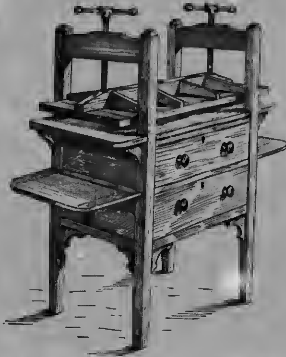
Fig. 1693.—General View of Cabinet Trousers Press.
