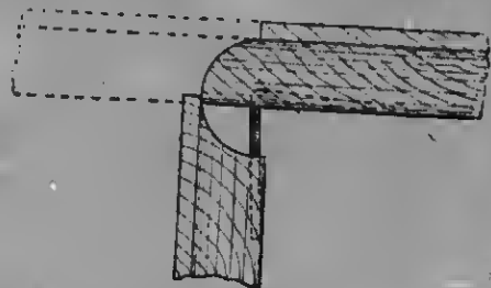
Fig. 41.—Joint between Table Top and Flap.
