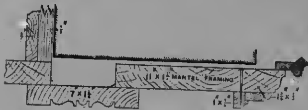
Fig. 705.—Horizontal Section through Mantel and Pilaster.
