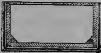
Fig. 1988.—Horizontal Section through Clock Case Base.
