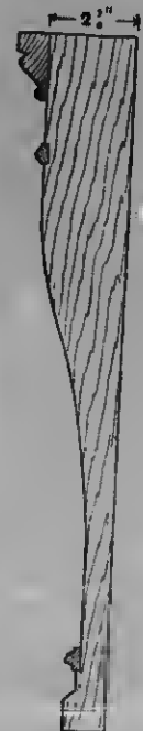
Fig. 182.—Section of Pilaster for Overmantel.
