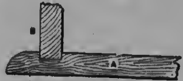
Fig. 664.—Section showing Washstand Sidepiece let into Grooved Top.
