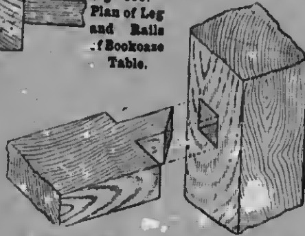
Fig. 961.—Joint of Leg and Shelf Rail of Bookcase Table.
