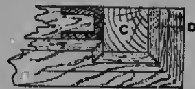
Fig. 1632.—Horizontal Section through Upright of Inlaid Frame.
