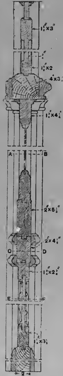
Fig. 1272.—Vertical Section of Hall Screen on Line G H (Fig. 1268).
