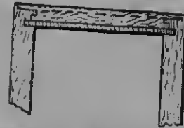
Fig. 1451.—Part Horizontal Section of Box with Secret Drawer.
