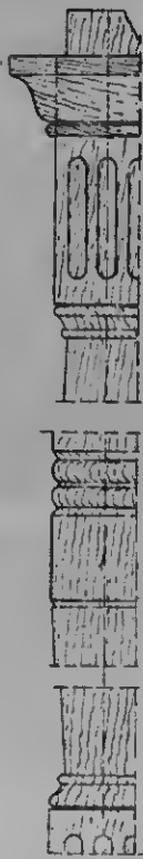
Fig. 1273.—Inner Stile or Column of Hall Screen.
