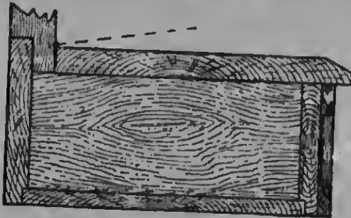
Fig. 1594.—Vertical Cross Section through Glove-box of Mirror.
