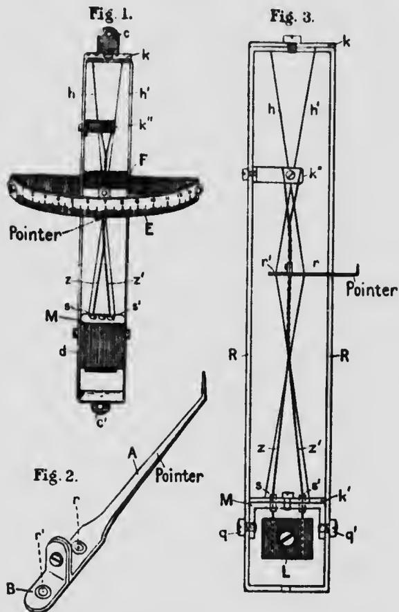
The two horsehairs (*h, h'*) that are used, are stretched tight by a torsion clamp (*Z, Z', and L*), which also carries the pointer; the position of the pointer varies with the length of the hairs, which,
