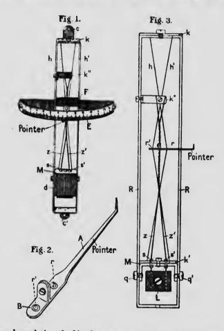
The two horsehairs (h, h') that are used, are stretched tight by a torsion clamp (Z, Z', and L), which also carries the pointer; the position of the pointer varies with the length of the hairs, which,
