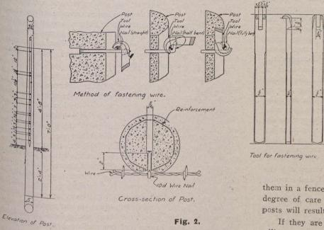
wire up close to the post. A tapered strip is now attached to the outside of the mould under the heads of the pins. It is of such a thickness that the offset in the holes is a uniform distance from the grooved side of the post and all nails project the correct distance to insure proper fastening of the wire.
