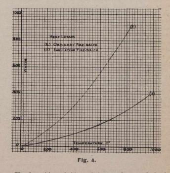
The first object of this work is to make a study in the quickest way possible of the heat insulating properties of various kinds of brick used in building furnaces and get some notion of the amount of heat lost with such materials. The ultimate object in view is the production of a heat insulating article, the cost of which will be less than that of the watt-hours uselessly dissipated through furnace walls.
