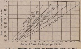
Fig. 5.—Results of Tests on Inspector Type of Pop Safety Valve.
