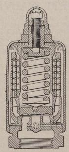
Fig. 6.—Muffled Locomotive Pop Safety Valve as Now Made.
