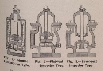
The additional lift due to the yielding of the metal because of the presence of steam pressure on the under side of the valve was determined in each case by placing the valve in a testing machine and subjecting it to a load corresponding to the steam pressure, the movement of the valve with relation to its seat being measured by a micrometer caliper.
