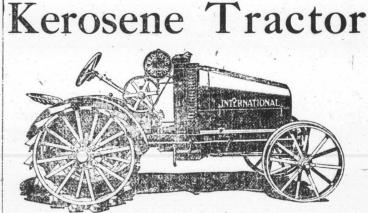
8-16 International-Valve in head Motor, THROTTLE GOVERNOR regulates fuel to load, friction Clutch Pulley.
