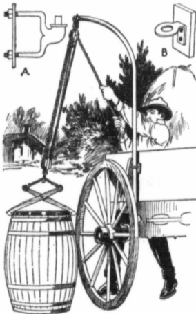
Wagon Crane Made of 2 Length of Gas Pipe with a Block and Tackle Attached
