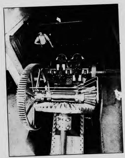
Cutter-head Engine, Hydraulic Dredge, No. 7.
