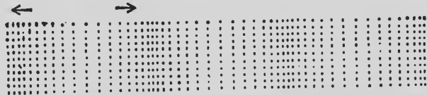
"The particles of air move backwards and forwards in forming the waves which produce sound" (p. 257).
