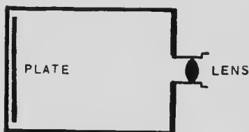
Diagram of photographic camera. Note the lens in front and the plate at the back.
