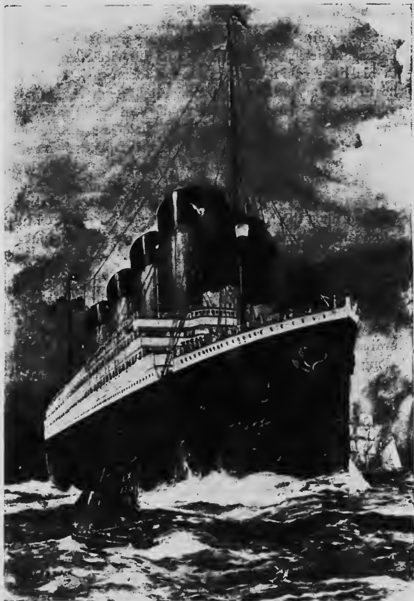
"Crossing from the Old Country" (p. 254). Note the two long wires stretching from mast to mast: they are the "ear" of the ship, and catch the electric waves of wireless telegraphy.
