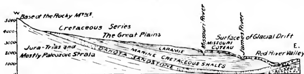
FIG. 33. Section from the Rocky Mountains to the Red River Valley, showing the water supply of its saline artesian wells. Horizontal scale 150 miles to an inch.
