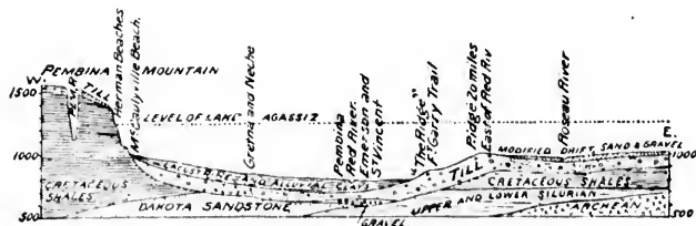
FIG. 6.—Section across the Red River Valley on the international boundary. Horizontal scale, 20 miles to an inch; vertical scale, 1,000 feet to an inch.
