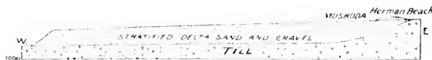
FIG. 14.—SECTION ACROSS THE DELTA OF THE BUFFALO RIVER. (The scale is in feet, half an inch to a mile.)
