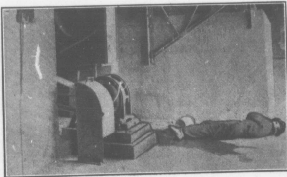
The result of using water to extinguish a fire in a motor.
