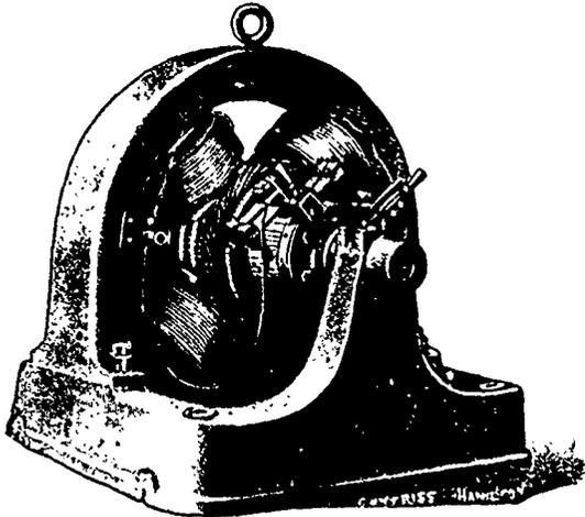
is perfectly symmetrical and balanced. The commutator is massive, made from the best copper, and wholly insulated with mica. Mechanically, the machine is unsurpassed. The armature is built on an open-work hub, which allows of thorough ventilation, and the commutator is directly keyed to same hub, the two forming a unit independent of the shaft, thus eliminating all strain at the armature leads, which often obtains in some types of machine by commutator working loose on the shaft.
