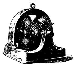
is perfectly symmetrical and balanced. The commutator is massive, made from the best copper, and wholly insulated with mica. Mechanically, the machine is unsurpassed. The armature is built on an open-work hub, which allows of thorough ventilation, and the commutator is directly keyed to same hub, the two forming a unit independent of the shaft, thus eliminating all strain at the armature leads, which often obtains in some types of machine by commutator working loose on the shaft.
