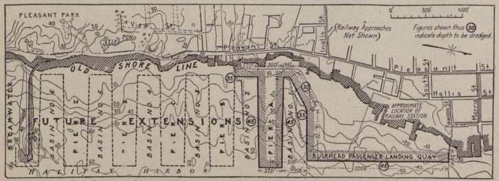
Fig. 5.—Layout of Quay and Piers and Location of Railway Terminal at Halifax. (Drawing by courtesy Engineering News.)
