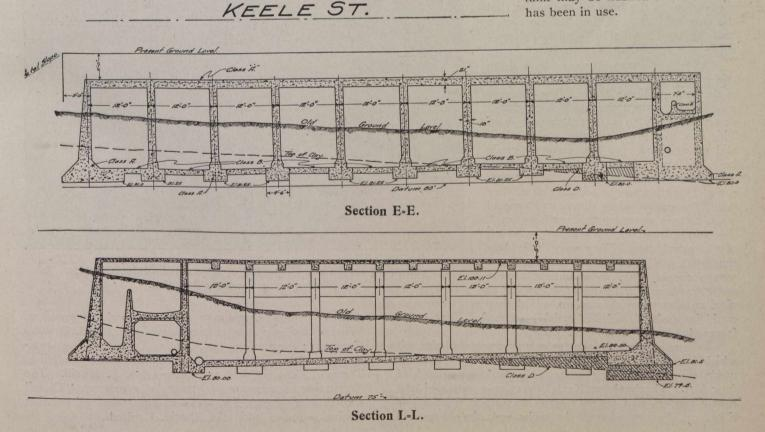
Construction.-The ground on which the tanks were built was composed of sand on the surface, which, in small areas, formed pockets. The sub-soil was hard, blue clay. Trenches were excavated by hand for the west wall and the western third of the north wall. This part was built first because the ground was low at this side. When these walls were built, and the concrete sufficiently hardened, they were used as a retaining wall for the next material
