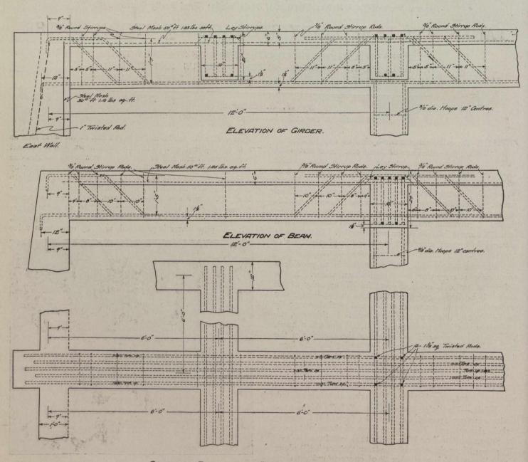
SECTIONAL PLAN THROUGH BEAM AND GIRDER.
