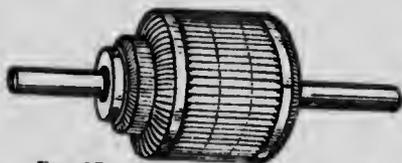
FIG. 97 A MODERN COMMUTATOR
