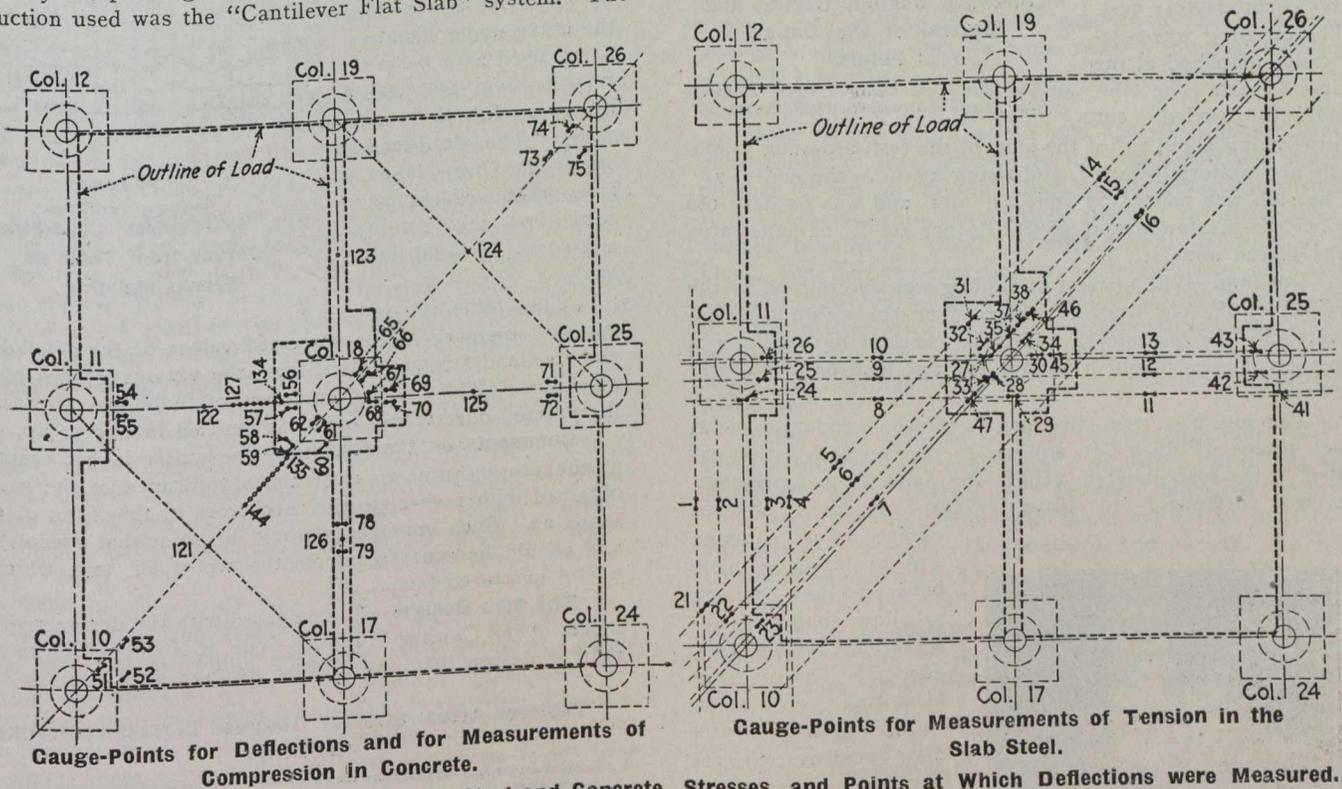
**Fig. 1.—Locations of Gauge Lengths for Steel and Concrete**
