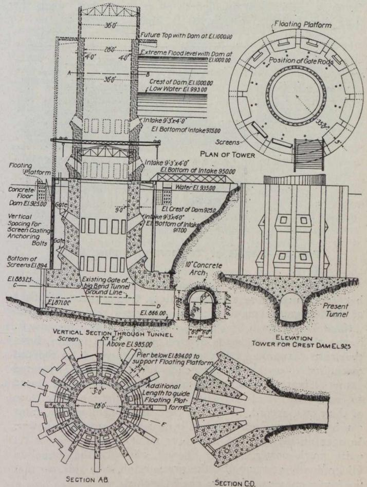
**Fig. 1.—Details of Tunnel Intake Tower.**
