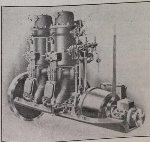
Fig. 5.—Direct Reversible Marine Engine.
