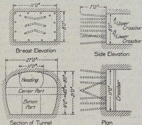
Fig. 1.—Scheme of Drilling Heading.
