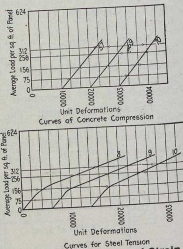
Fig. 4.—Typical Load-Strain Curves from Tests in Franks Building.
