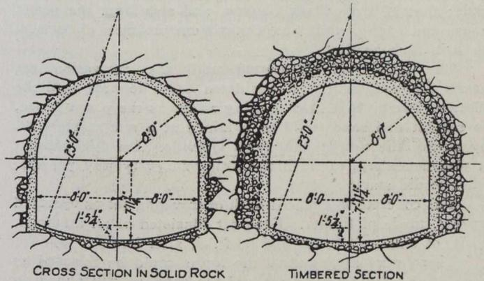
Fig. 4.—Typical Sections of New Tunnel.
