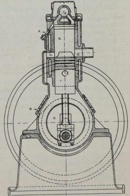
Fig. 6.—Section Through Direct Reversible Marine Engine.
