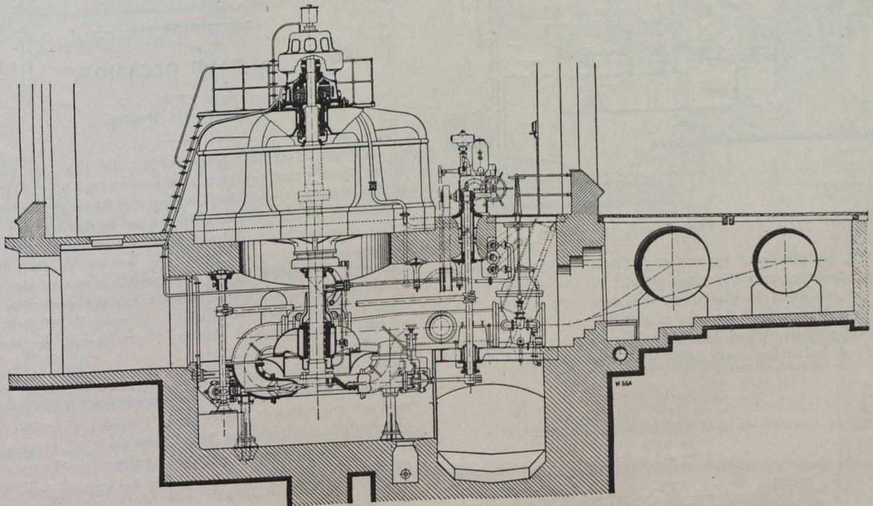
Fig. 1—Longitudinal Section through 10,000 H.P. High-pressure Turbines.
