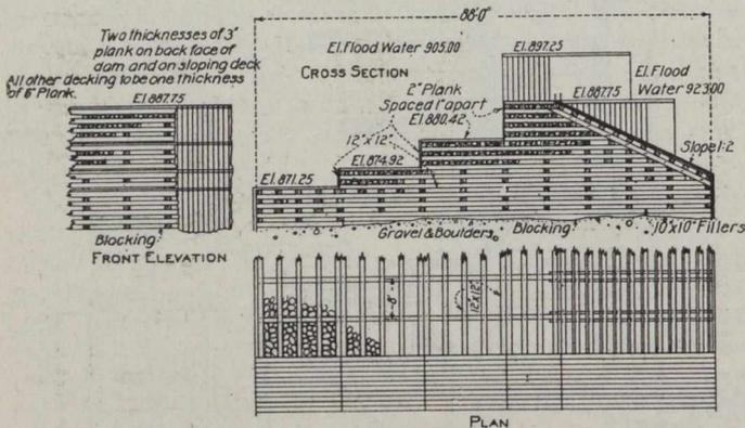
Fig. 2.—Details of Temporary Timber Dam.
