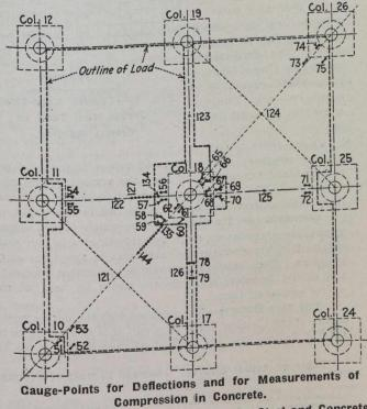
Fig. 1.—Locations of Cauge Lengths for Steel and Concrete
