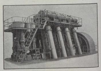
Fig. 4.-Four-Cylinder Two-Cycle 2,400 b.h.p. Engine.
