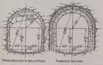
Fig. 3.—Typical Sections of Enlarged Tunnel.
