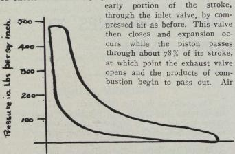
Fig. 2.-Indicator Daigram of Four-Cycle Diesel Engine.
