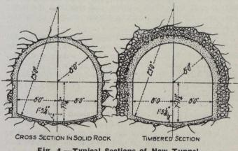
Fig. 4.- Typical Sections of New Tunnel.
