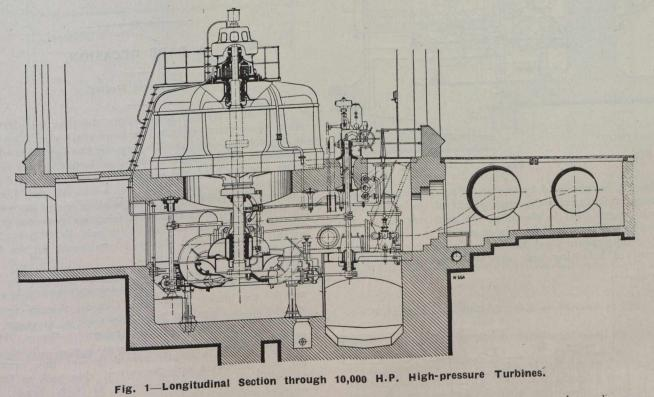
Each of the two pipe lines delivers the necessary amount of water required by two high-pressure impulse wheels, each capable of developing an output of 10,000 horse-power when running at 300 revolutions per minute. However, in accordance with the specifications, each of the wheels is designed so as to yield a maximum power, at full
