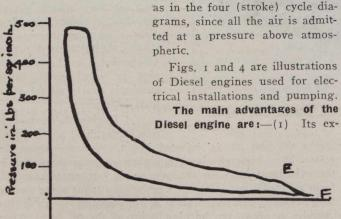
Fig. 3.-Indicator Diagram of Two-Cycle Diesel Engine.
