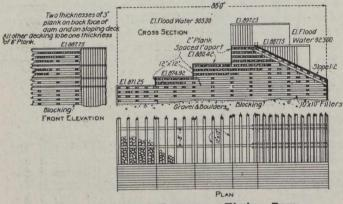
Fig. 2.—Details of Temporary Timber Dam.
