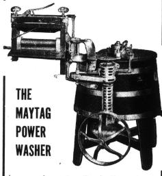
in general construction is the same as the Multi-Motor. It has a pulley so it can be driven by a separate engine.
