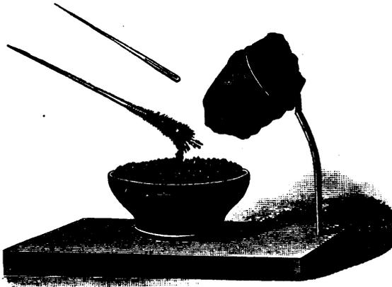
FIG. 10.—MAGNETIZATION BY LOADSTONE.
