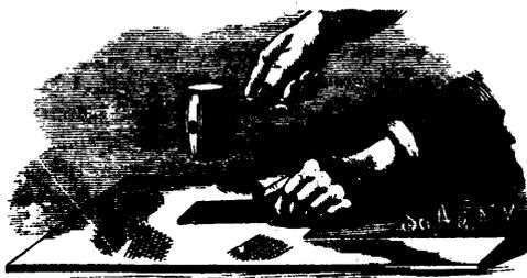
FIG. 2.—ROUGHENING THE PLATE.
