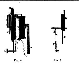
to these tubes are metal pins, e,  $e^{2}$ , against which the needle, n, strikes. The two tubes are made of different thicknesses of metal, so that they emit different notes.
