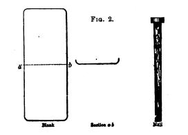
NAILS FROM TIN-SCRAP. BLANK AND FINISHED NAIL. FULL SIZE.
