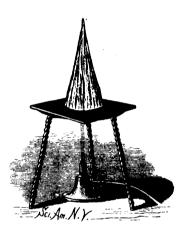
FIG. 5.—SENSITIVE FLAME WITH GAS AT ORDINARY PRESSURE.
