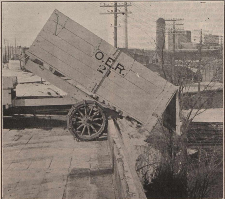
Snow Dumping Motor Truck, Ottawa Electric Railway.
