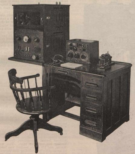
Wireless telegraph set for steel steam drifter, built by Marconi Wireless Telegraph Co.
