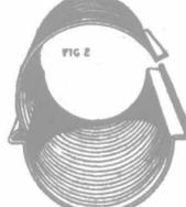
ribs, engage easily, as you see in Fig. 2. The joints between one length and another are "broken"—no over-lap reaches more than half-way round the culvert's diameter; and this is possible with NO OTHER metal culvert made. It is a most valuable feature, for it reduces the chance of leakage to the very least minimum.
