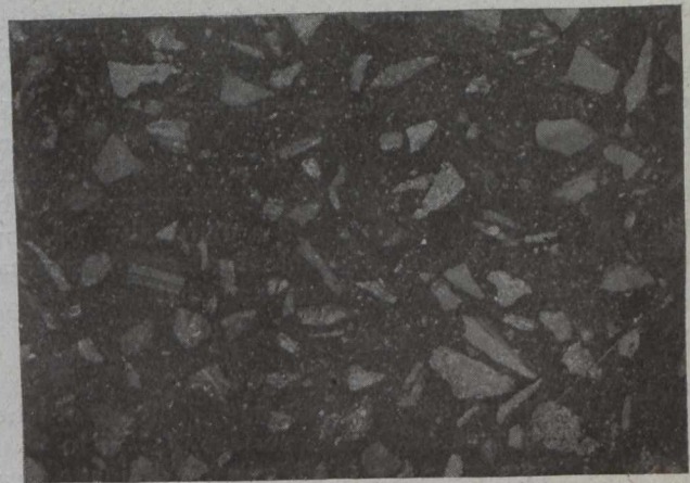
Actual Size Photograph of Surface of Stone-filled Sheet Asphalt Pavement, as Laid in Montreal, After Being Rubbed Down on Marble Bed.
