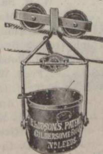
61—Rope Bucket, with R. H.'s Patent Catch for Wire Rope Tramways
