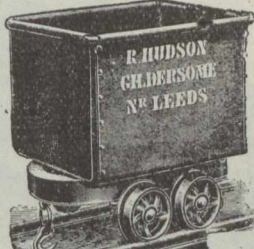
70—R. H.'s Patent Steel Mining Wagon
