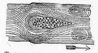
The two currents are then deflected from the shores toward the island, which is thereby curtailed in its lower parts, and at its extremity contracted almost to a point. The two currents unite below, and form a deep channel. At the head of the island the water is shallow. The largest and oldest timber stands on the lower end, and  $\kappa \beta$
