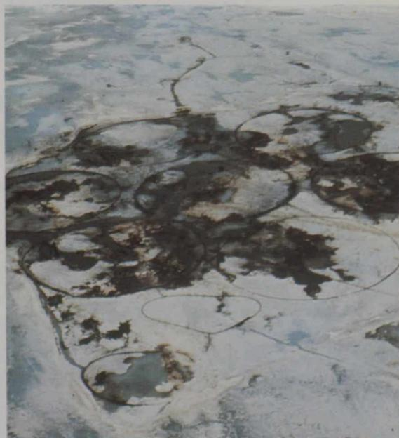
*Oil rising to the surface in Balaena Bay: the circular pattern is caused by containment booms under the ice.*
