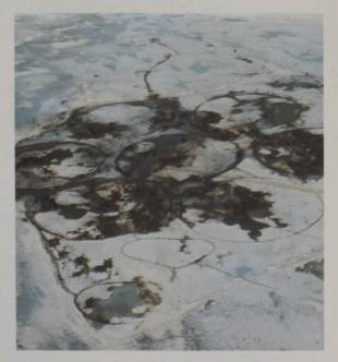
Oil rising to the surface in Balaena Bay: the circular pattern is caused by containment booms under the ice.
