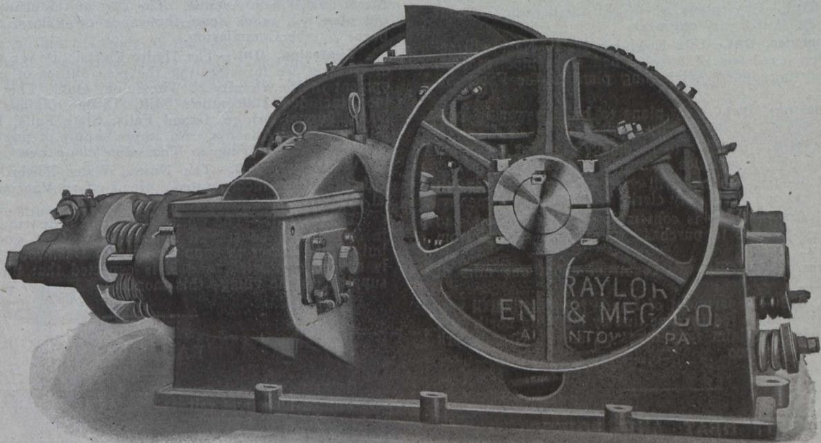
Owing to the automatic lateral shifting device, you get the maximum tonnage per set of shells and consume the minimum horse power; for all *corrugating* and *flanging* of the roll shells are eliminated by this strong, simple and positive device.
