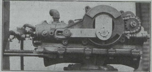
Gasoline Rock Drill Has Double Piston
