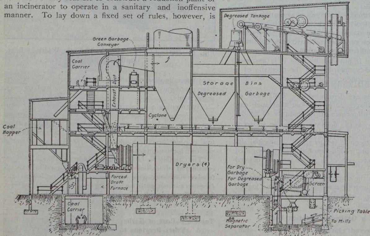
**Fig. 2.—Longitudinal Section of Dryer Building, Chicago Municipal Reduction Plant**
