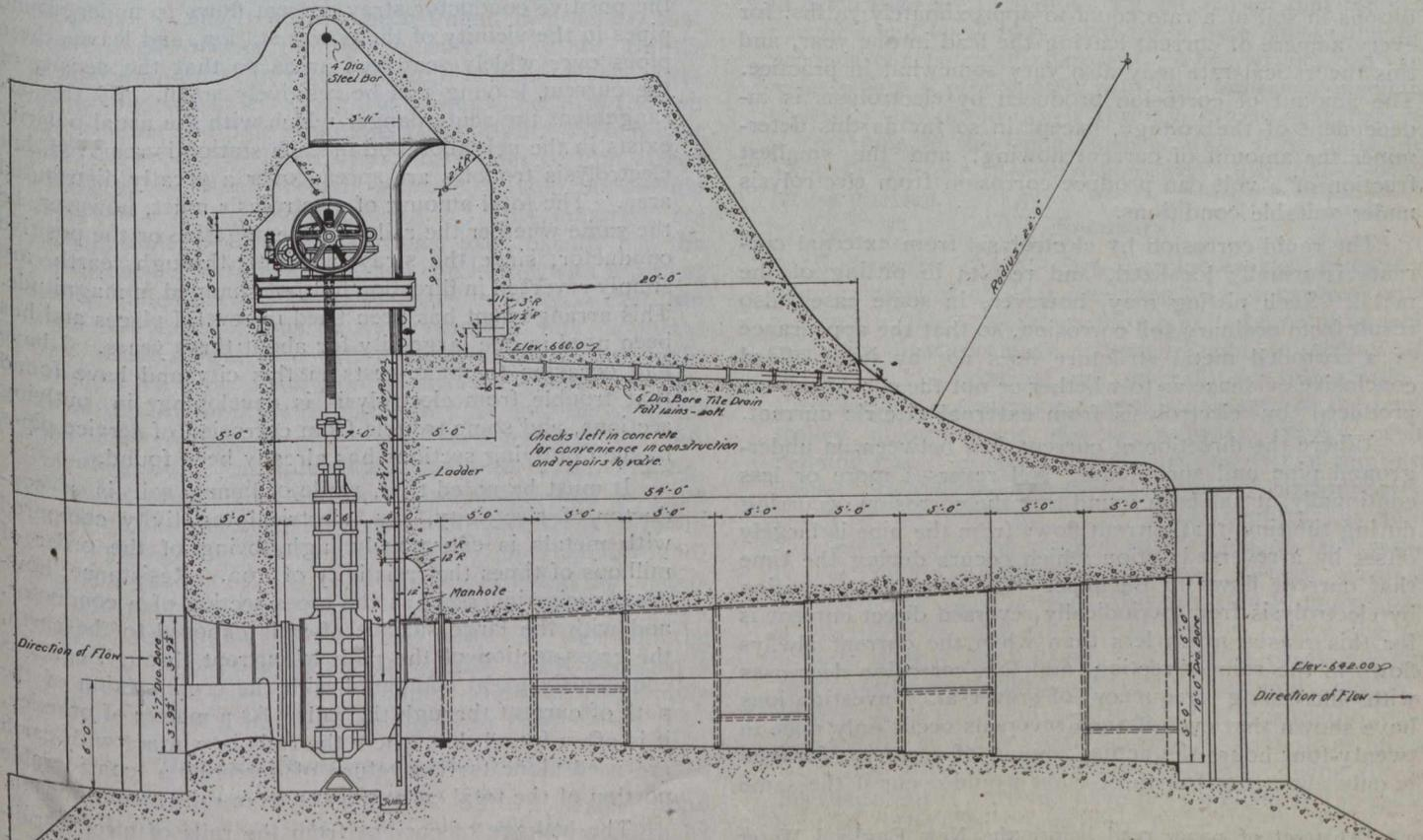
Fig. 5.—Side Elevation Showing Sluice Pipe and Sluice Valve and Arrangement of Operating Winch
