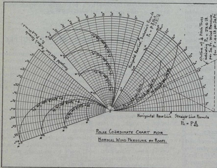
The values in the following table were calculated from the formulas given above and the Polar-Co-ordinate chart plotted from these values will be found very convenient for reading direct the normal pressure at any inclination.
