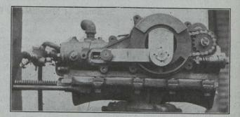
Gasoline Rock Drill Has Double Piston
