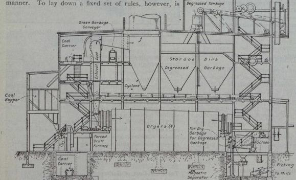
Fig. 2.-Longitudinal Section of Dryer Building, Chicago Municipal Reduction Plant
