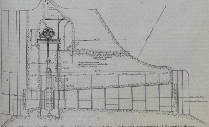
Fig. 5.-Side Elevation Showing Sluice Pipe and Sluice Valve and Arrangement of Operating Winch
