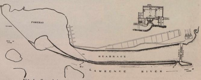
Fig. 1.—General Arrangement of Plant, and Cross Section of Power House.
