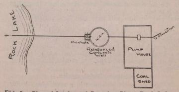
Fig. 3.—Plan of Intake and Pumping Plant, Rock Lake.
