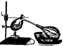
flask in a pan of cold water. Cover the flask with a cloth or with blotting paper, and pour cold water from time to time upon it. Place the retort upon wire-gauze on a ring of the retortstand, and boil the water. As fast as the
