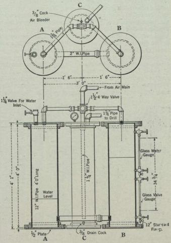
FIG. 1.-WATER DISPLACEMENT AIR METER FOR ROCK-DRILL TESTING.
