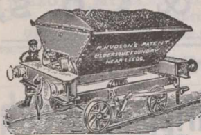
59—R. H.'s Patent 6-Ton Steel Double Side Tip Wagon, to work with ordinary Idy Wagons
