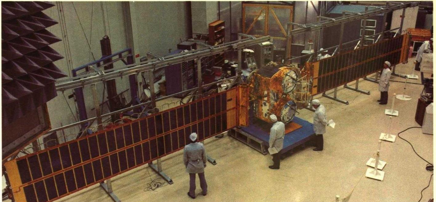
**HERMES** was a compact bundle (top left) when it was launched in 1976. Once in space, its arrays or sails unfolded accordion-style (top right). The arrays (bottom) have 27,000 solar power cells, which provide 1.2 kilowatts of power. The two large discs on the body are antennas.
