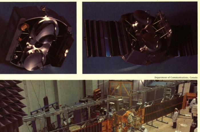
HERMES was a compact bundle (top left) when it was launched in 1976. Once in space, its arrays or sails unfolded accordion-style (top right). The arrays (bottom) have 27,000 solar power cells, which provide 1.2 kilowatts of power. The two large discs on the body are antennas.
