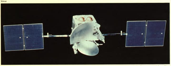
Anik B, Canada's newest commercial domestic communications satellite, uses technology developed by HERMES. It is the first commercial satellite to use both the 6/4-GH, and the 14/12-GH, bands.
