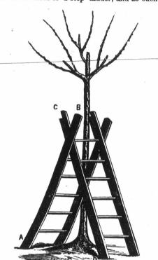
be used under and about small trees for gathering fruit, pruning or grafting. When straightened out so that the side c, D forms a continuation of A, B, it forms a long ladder, the point C striking against the upper round of the lower part. If desired, the two parts can be separated, making two short ladders. A useful size is about nine feet for each length.
