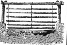
companying engraving is well adapted for the pur-The one at the top is made from poles of the desired length woven together with strong wire which, in turn, is secured to the overhanging pole As the water rises the poles float upon its surface and do not in the least impede its onward progress. | and not pedigrees.
