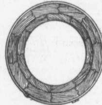
End view of Pipe and Coupling
