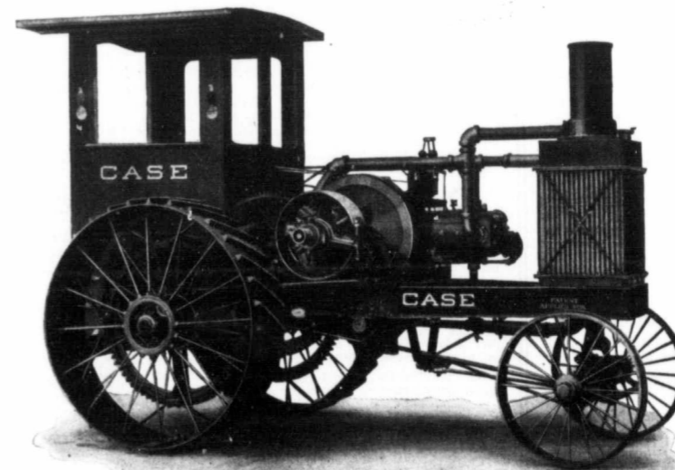
The 60 H. P. Oil Tractor burns kerosene, gasoline, naphtha or distillate.
