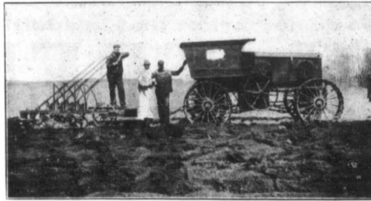
The Canadian Heer Tractor Plowing Near Stonewall, Man., Pulling a Cockshutt 4-bottom Engine Gang, soon as you have finished with it.
