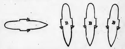
The manner of fixing the colored lights should be particularly attended to. They will require to be fitted each with a screen, of wood or canvas, on the inboard side, and close to the light, in order to prevent both being seen at the same moment from any direction but that of right shead to two points abaft the beam.
