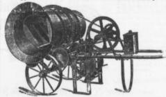
These machines are made to mix either continuously or in batches, and carr be operated either by Hand Steam or Gasoine Power.
