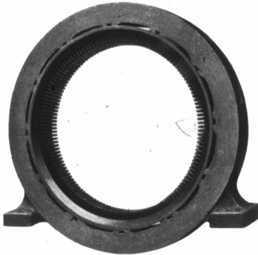
Fig. 4—Stator Core, Type G Generator
