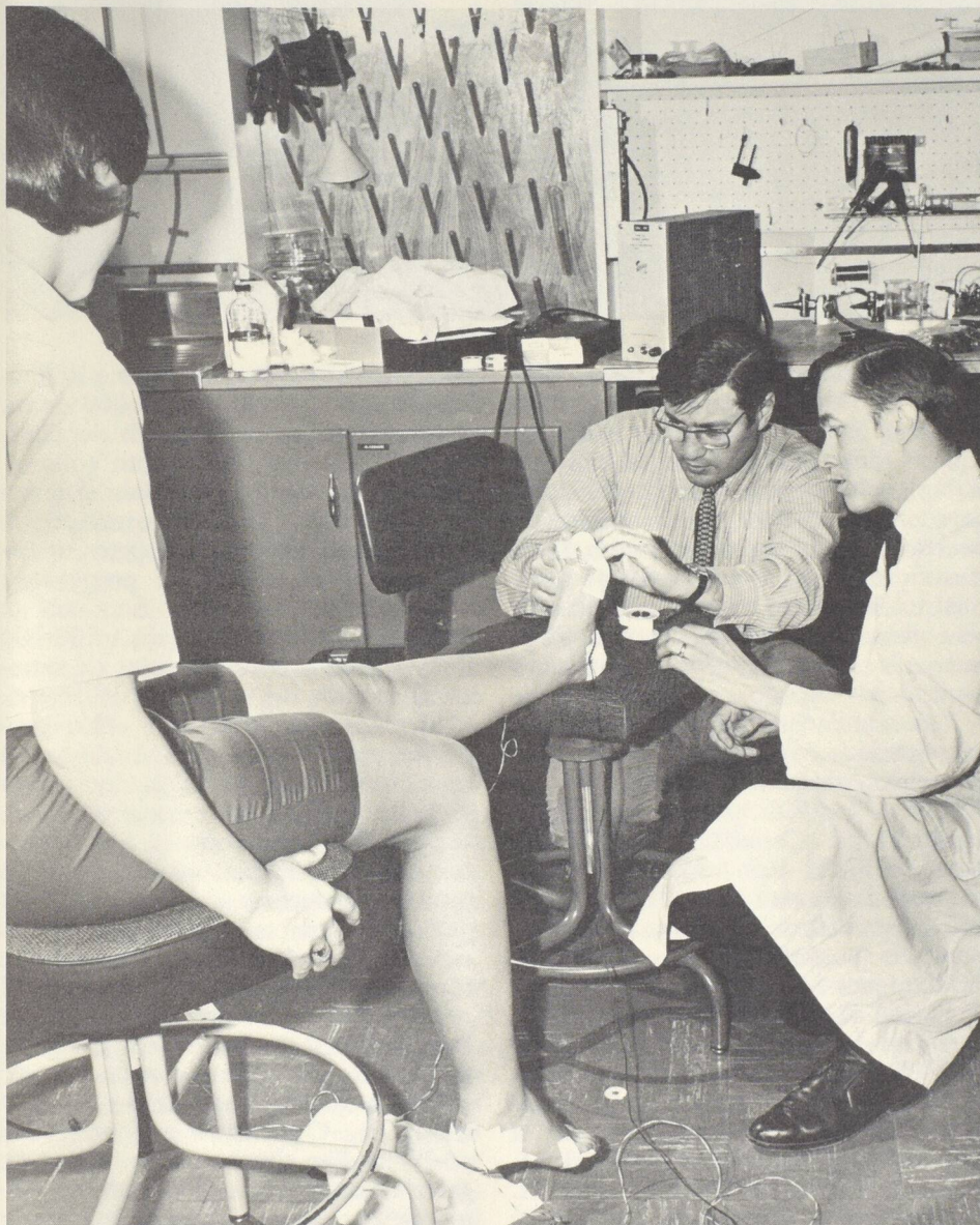
Dr. Morris Milner (left) and Arthur Quanbury attach footswitch electrodes to the foot of a subject at the start of a gait characteristics study.
