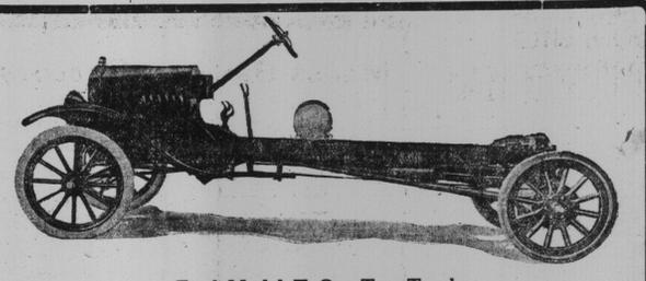
Ford Model T One-Ton Truck Can be equipped with any style of body to suit individual requirements. Standard equipment includes hood for motor, front fenders, stepping boards, two side-lights, two head-lights, one tail-light, horn and set of tools.
