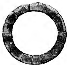
Horizontal Section, 20 feet circumference.
